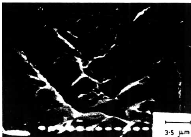
Fig. 1(d). Morphology of H 25 extruded at a shear rate of 1223 s -1 showing the periphery region.
