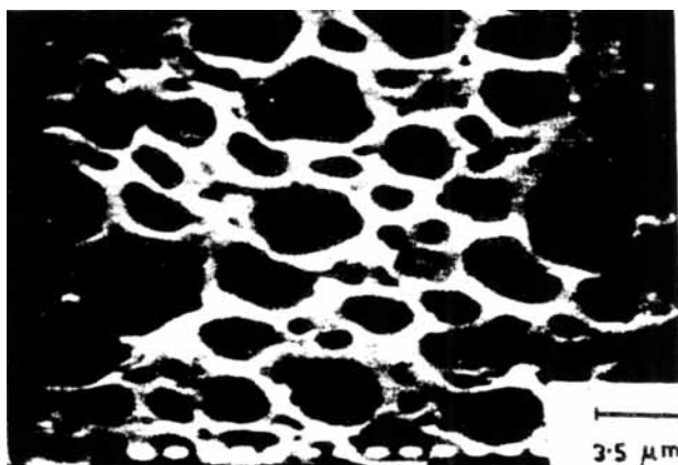
Fig. 2(a). Morphology of H_{50} extruded at a shear rate of 122 \text{ s}^{-1} showing the core region.
