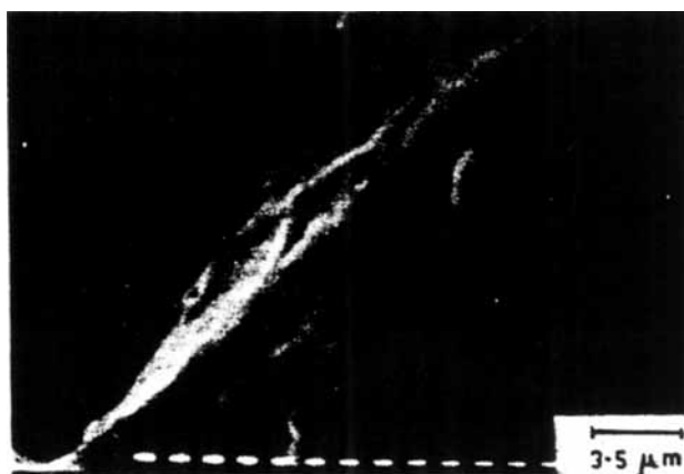
Fig. 2(d). Morphology of H_{50} extruded at a shear rate of 1223 \text{ s}^{-1} showing the periphery region.
